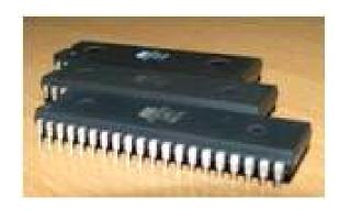
The AT89S52 is a superior CMOS 8-bit microcontroller, low-power, with 8K bytes of EPROM. These are components of AT89S52 microcontroller: 256 bytes of RAM, 8K bytes of Flash, , three 16-bit clock/counters, 32 info/yield pines , two information pointers, Watchdog clock. six hinder of two level construction modeling, serial port, oscillator . the AT 89C52 is effective MC which gives an adaptable and
