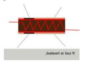
If the coil is heated up, SnO2 earthenware production will turn into the semi - conductor, so there are more portable electrons, which implies that it is prepared to make more present stream.
